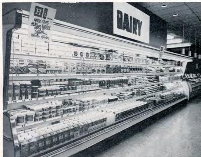
This five-tier, air-curtain dairy case is the latest and most efficient type available anywhere in the country.
